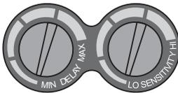
The operator may adjust clearing delay time with the **OPÓZNIENIE/DELAY** knob located on the filter cartridge near the **CZUŁOŚĆ/SENSITIVITY** knob. With this knob, you can set the filter reaction time between 0.1 s and 1.0 s.
